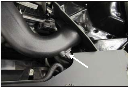
11. Reconnect the Mass Air Flow sensor. Slide the locking tab back into the connector.
