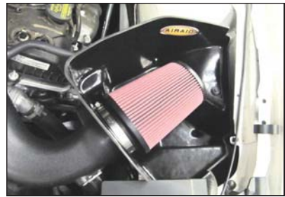
12. Install the Airaid Premium Filter (#1) onto the Intake Tube and tighten the hose clamp.
