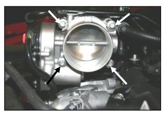
**3.** Remove the four bolts that secure the throttlebody to the intake manifold and set aside. They will not be reused.
