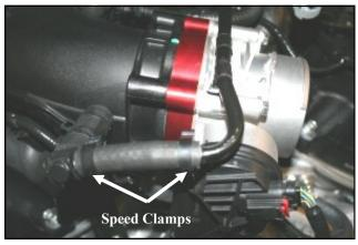
**5.** Remove the factory breather hose and spring clamps, and replace them with the supplied Breather hose and Speed clamps. Re-torque the throttlebody bolts in a X pattern, to Factory specs.
