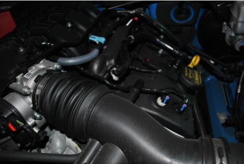
3. Now cut the tape holding the second breather tube to the plastic mount located on top of the throttle body (as shown below.)
