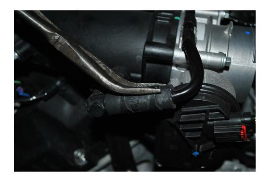
5. With the 2nd breather tube out you can now remove the other squeeze clamp and remove hose from 90 degree fitting, set the hose and 2 clamps aside as they will not be reused.
