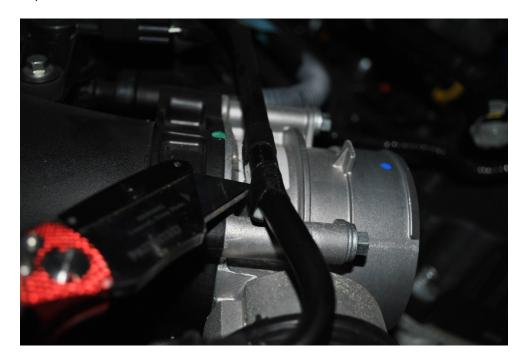
4. Now remove the first squeeze clamp on the second breather tube with needle nose pliers or channel locks (as shown below.) Slide the clamp off of the hose and over the breather tube. You can now pull the tube out of the hose.
