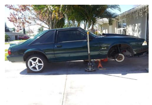
2. Now that both wheels are up off the ground and safe, feel free to turn the wheel toward the side that you are going to be working on. Just do one side at a time.
