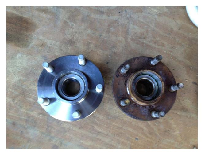
8. Place the new wheel hub on to the spindle , Take the new hub nut and start it by hand. Take the 36mm socket and torque wrench and tighten the new hub nut to the torque of 221 to 295ft-lbs
