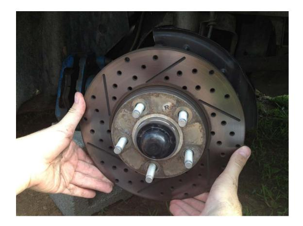
12. Replace the rotor back onto the new hub assembly you have just installed.
