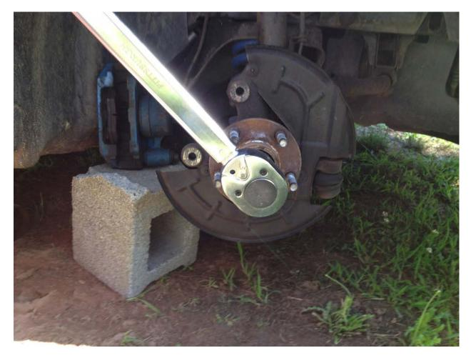
7. Clean the spindle on the car with a rag. Lubricate the spindle with wheel baring grease
