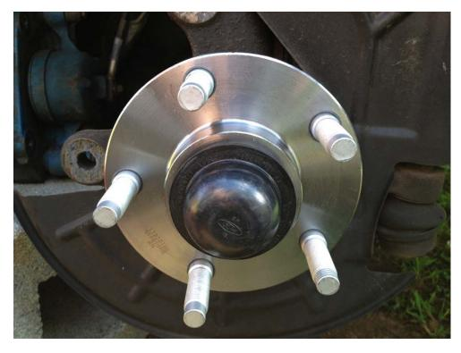
10. With a small piece of 2x4 place it on the edge of the hub and easily tap with a hammer all the way around the dust cover to get it started (use wood so it does not bend or damage the dust cover)
