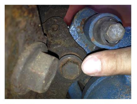
**3.** Place brakes caliper either on a cinderblock or hang it the proper height so not to damage the brake line).
