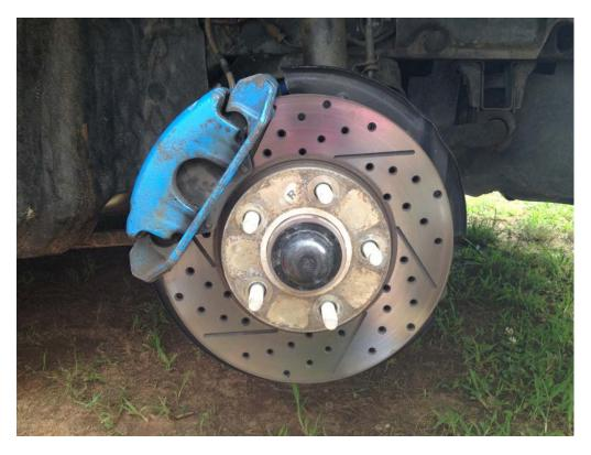
13. Take the brake caliper and slowly slide over the rotor line up and start the 2 bolts that hold the caliper into place. Torque the bolts to (1997 and earlier) 65ft-lbs (1998 and later) 23ft-lbs Re-install the wheel and torque lug nuts to 85 to 105ft-lbs. Remove the jack stands. Lower the car.
