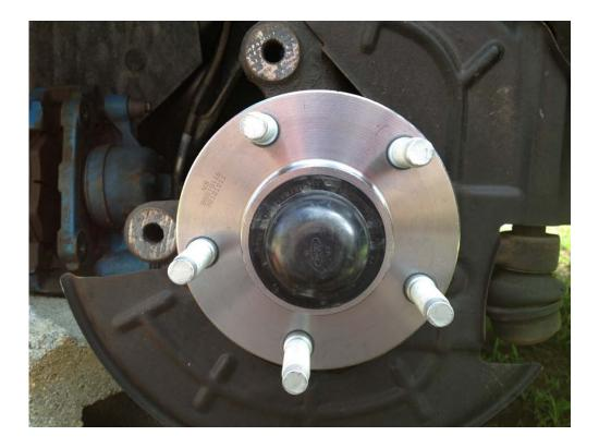
11. Replace the rotor back onto the new hub assembly you have just installed
