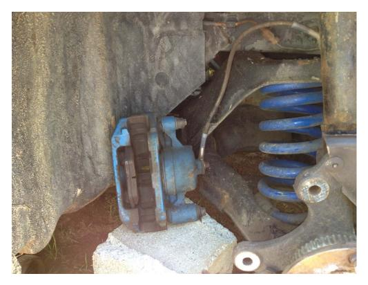
4. Remove the rotor, Place it to the side
