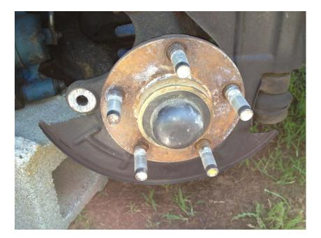
5. Take flat head screwdriver and easily tap it in around the dust cover with the hammer to remove it from the hub (the dust cover is a onetime use item, so you will have to replace it with a new dust cover each time)
