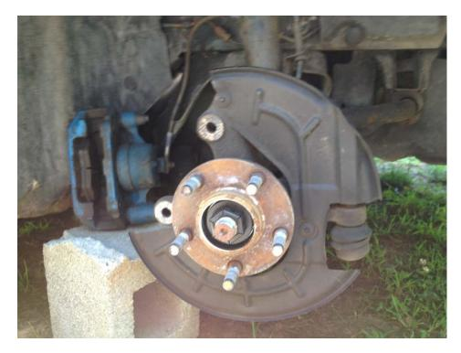
6. Using the 36mm socket remove the hub nut (this is a onetime use hub nut) Remove wheel hub
