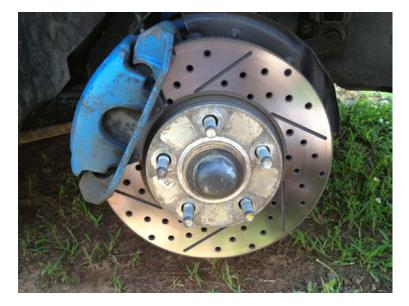
2. Use 15mm socket to remove the brake caliper (2 bolts on back of caliper)
