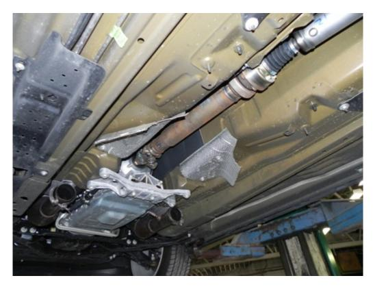
4. Remove rear H-pipe clamps from factory H-pipe using a flathead screwdriver to release the tabs and place on Boss 302 H-pipe.
