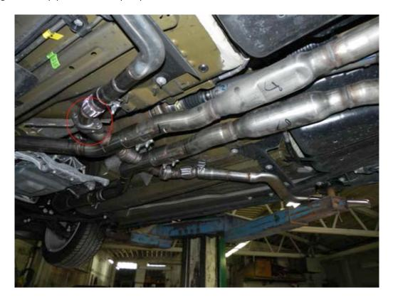
7. Take the supplied 15mm bolt from the package and line the side exhaust outlet up to the hole under the body and tighten it, repeat for the other side. (Convertible models see note)
