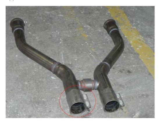
5. Install new Boss 302 H-pipe. To make the installation smoother, I chose to place the rear exhaust clamps on the mid-pipe and slide them forward onto the H-pipe. Align forward ball socket and tighten clamps down. Slide the rear clamps forward until they clip on and tighten them down. You are now done with the hard part.
