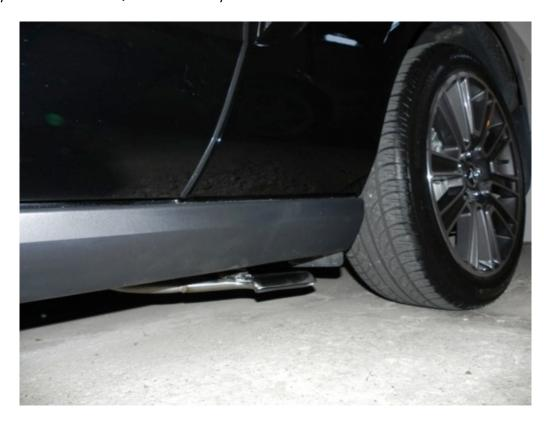
In order to secure the outlet end of the side exhaust, you have to remove the bolt from the convertible brace (See Photo Below) and replace it with a longer one and a spacer (See Second Photo Below). I used an M10-1.50x70mm 15mm bolt purchased from the local hardware store along with a 1" spacer. It will make the outlets sit lower than on the coupe, but it does not interfere with function.
