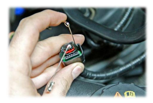
Push the second safety pin down and you will feel it slide down. Do not force it! DO ONLY ONE AT A TIME so you won't get the wires mixed up.
