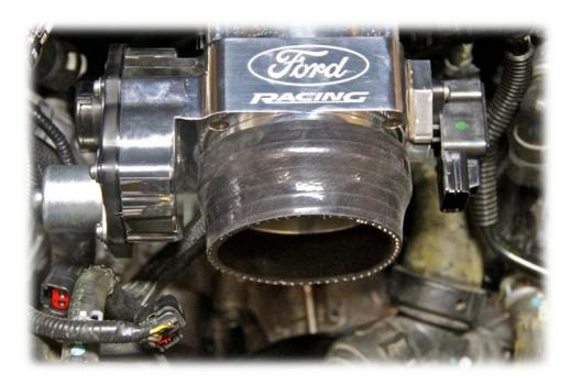
8. The ford racing manifold comes with a new throttle position sensor as seen below
