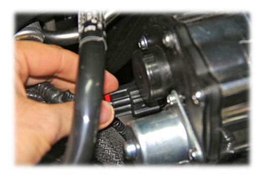
10. This part is tricky so PAY ATTENTION. The stock throttle position sensor WILL NOT connect to the new throttle position sensor as seen below
