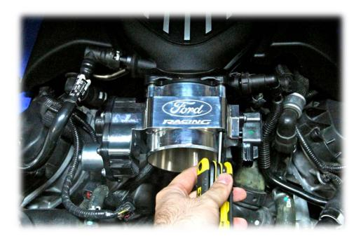
7. Slide on the silicone coupler onto the ford racing throttle body. This will not be easy. If you can purchase one that will go on easier then by all means do so.
