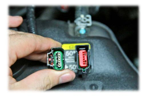
You will have to take off the red plastic cover that is on the inside of the stock throttle position sensor (use a small thin screw driver to remove it)
