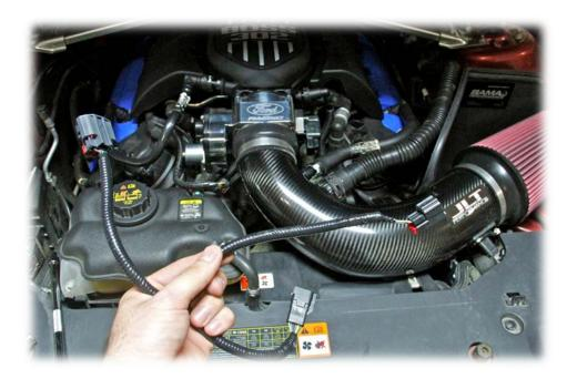
Before connecting the intake to the silicone coupler; using the new throttle position sensor, plug in the "big gray plug" onto the throttle body, and secure it with the red clip that is attached
