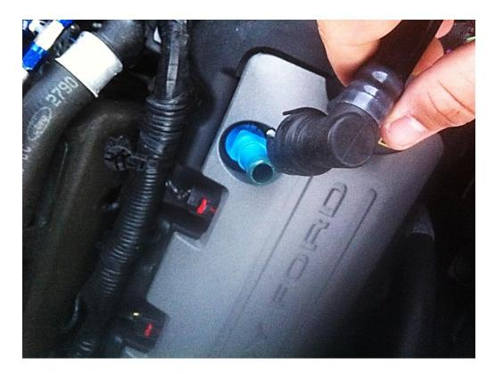
6. Remove the Spark Plug Cover by simply pulling off.
