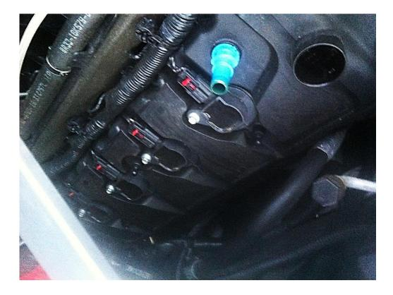
7. Remove the 5/16" bolt holding down the coil and then remove the coil. Check coil to make sure there are no tears, no burn marks, or oil on them. This would also be a good time to upgrade your coils.
