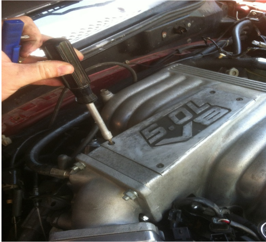
Photo 3: Torx T-20 for plenum cover. 6 bolts (1/2") secure upper plenum to lower.
