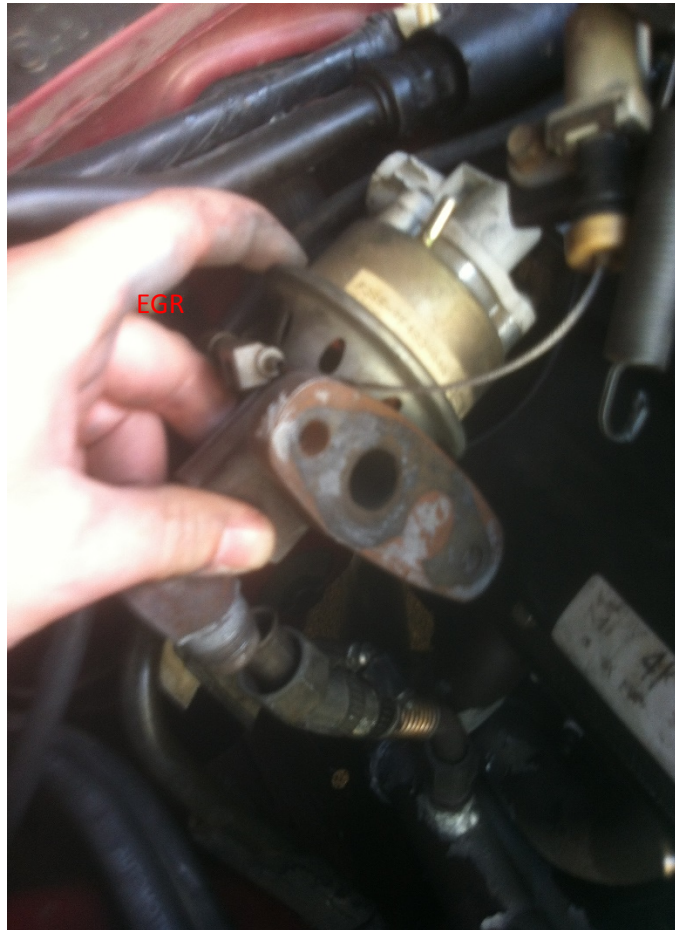
Photo 2: 94-95' Models have EGR plumbed directly into passenger exhaust manifold.
