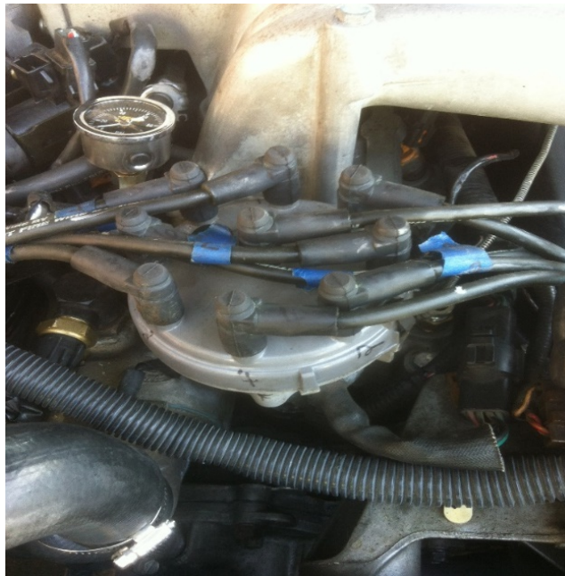
Photo 8: Labeling distributor cap and plug wires for convenience later on.
