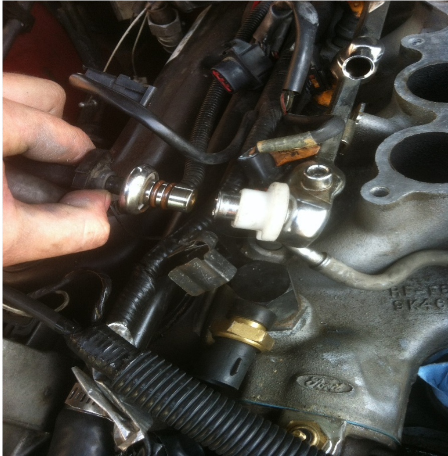
Photo 6: Using disconnect tool to unhook fuel lines. Don't lose metal snap locks.
