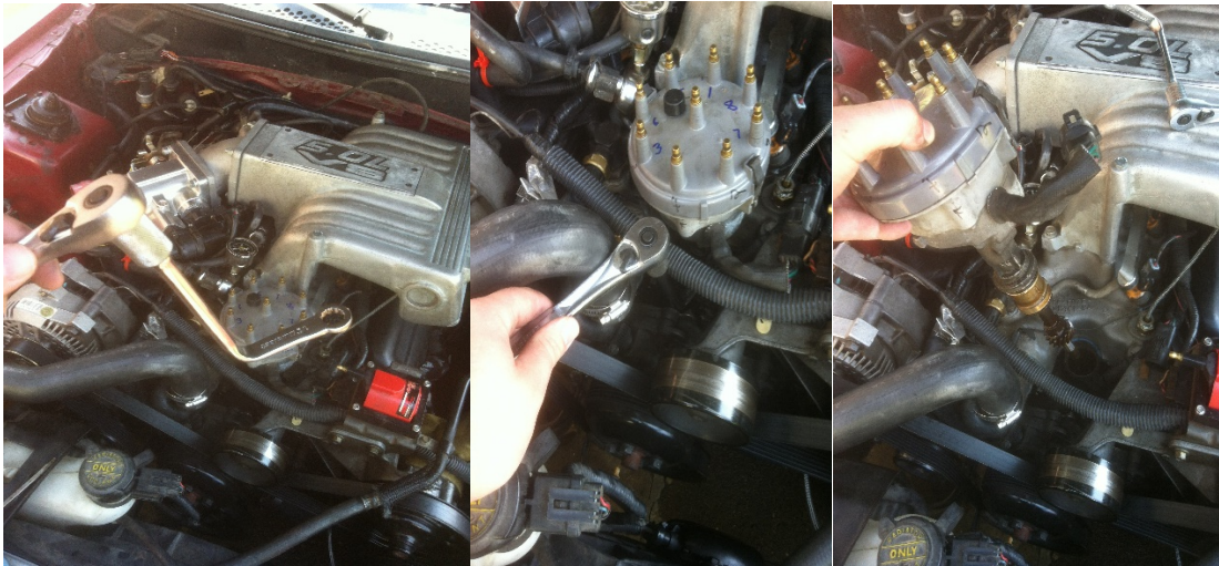
Step 22. Photo 9: Using distributor wrench to remove \frac{1}{2} " bolt securing distributor.
