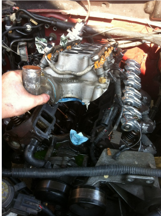
Photo 11. Prying the lower intake manifold up to break old gasket seals.
