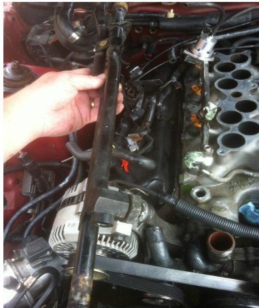
Photo 5: Coolant crossover tube 94-95' models. Fox will have two connections to lower intake as well as small coolant line that runs through EGR spacer on upper plenum
