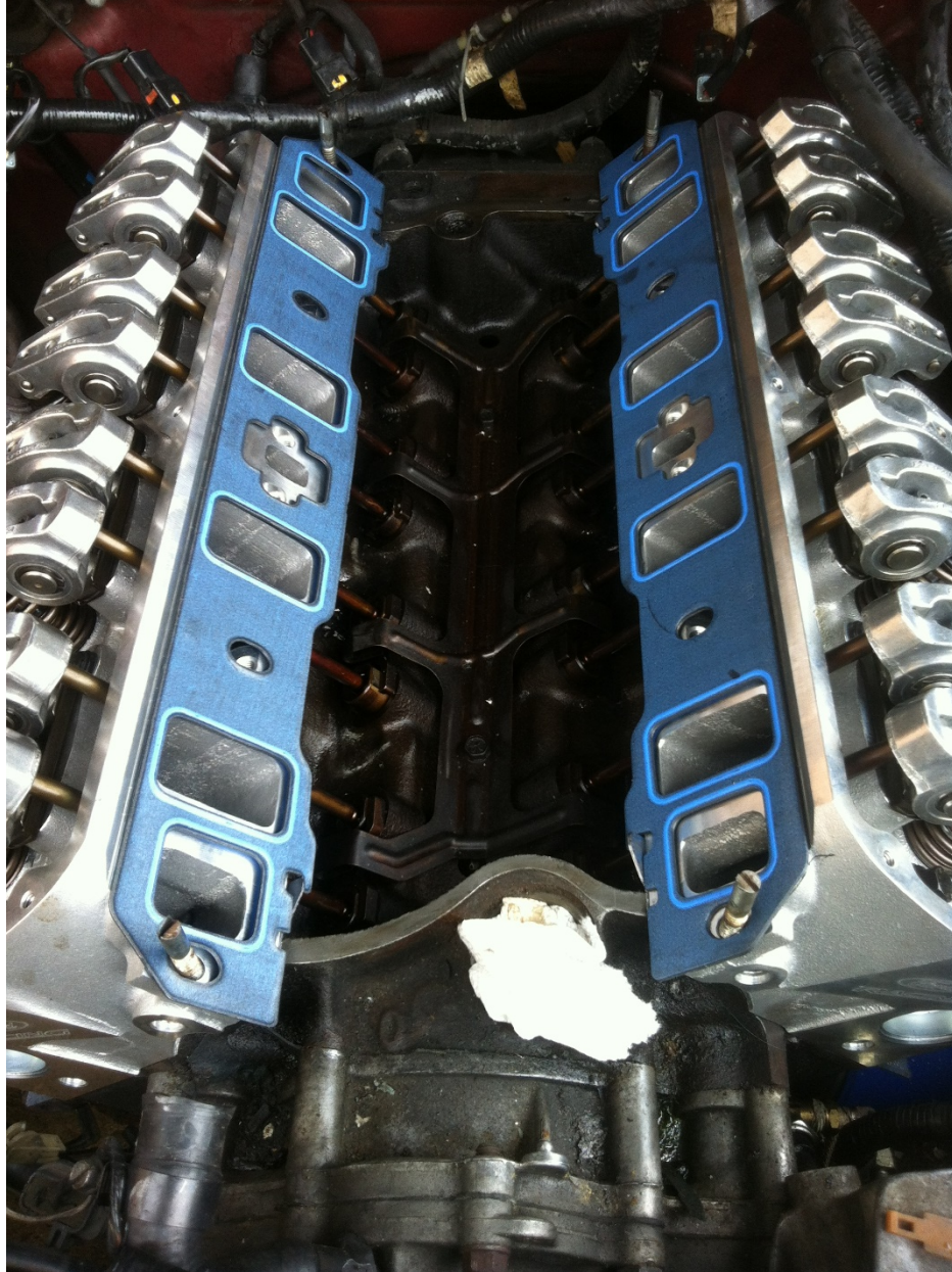
Photo 13: Always check port alignment of your gaskets between the cylinder head and intake, test fit your intake without bolting it down first.
