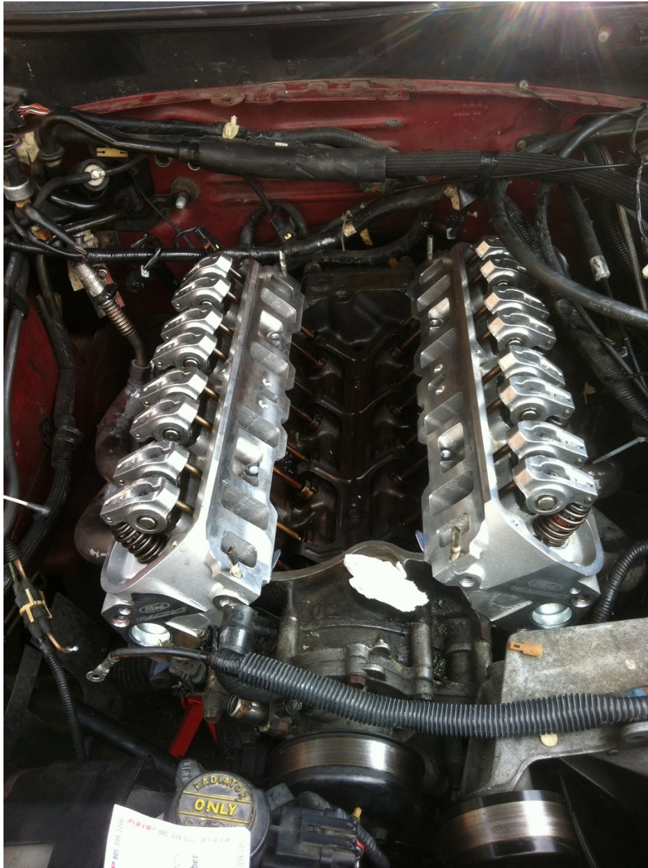
Gasket surfaces prepped and ready to place gaskets.
