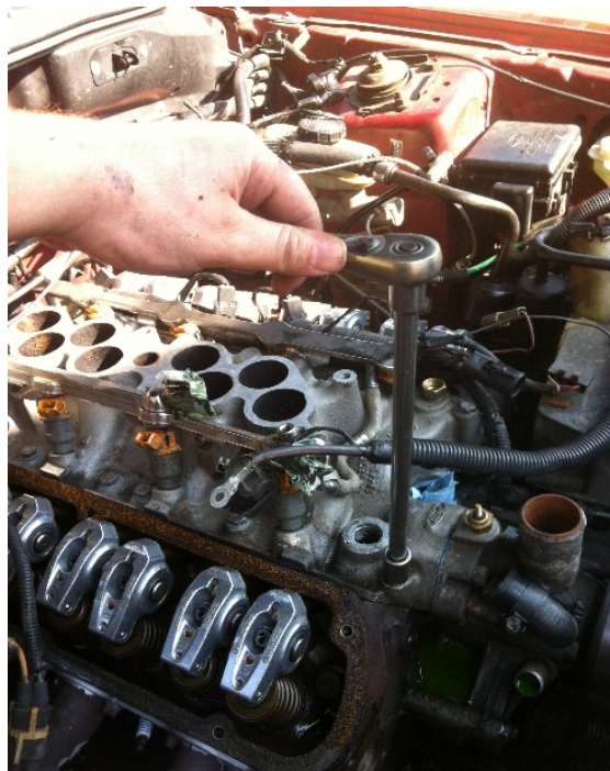
Photo 10. Unbolting the 12 lower intake manifold bolts.
