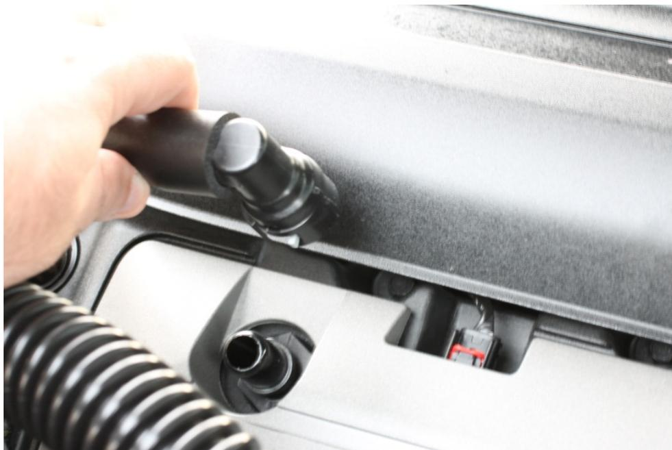
8. Remove the stock Coil Cover by gently unsnapping it from the mounting points.
