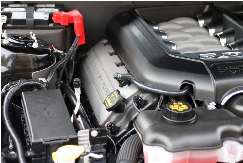
3. Remove the Positive Crankcase Ventilation Tube (PCV Tube). At the base of the tube, you will find a gray ring with a small release pin on it. To remove, simply slide the release pin along the side of the tube, and pull the PCV Tube towards you. Use the screwdriver to gently slide the pin if your fingers cannot reach.
