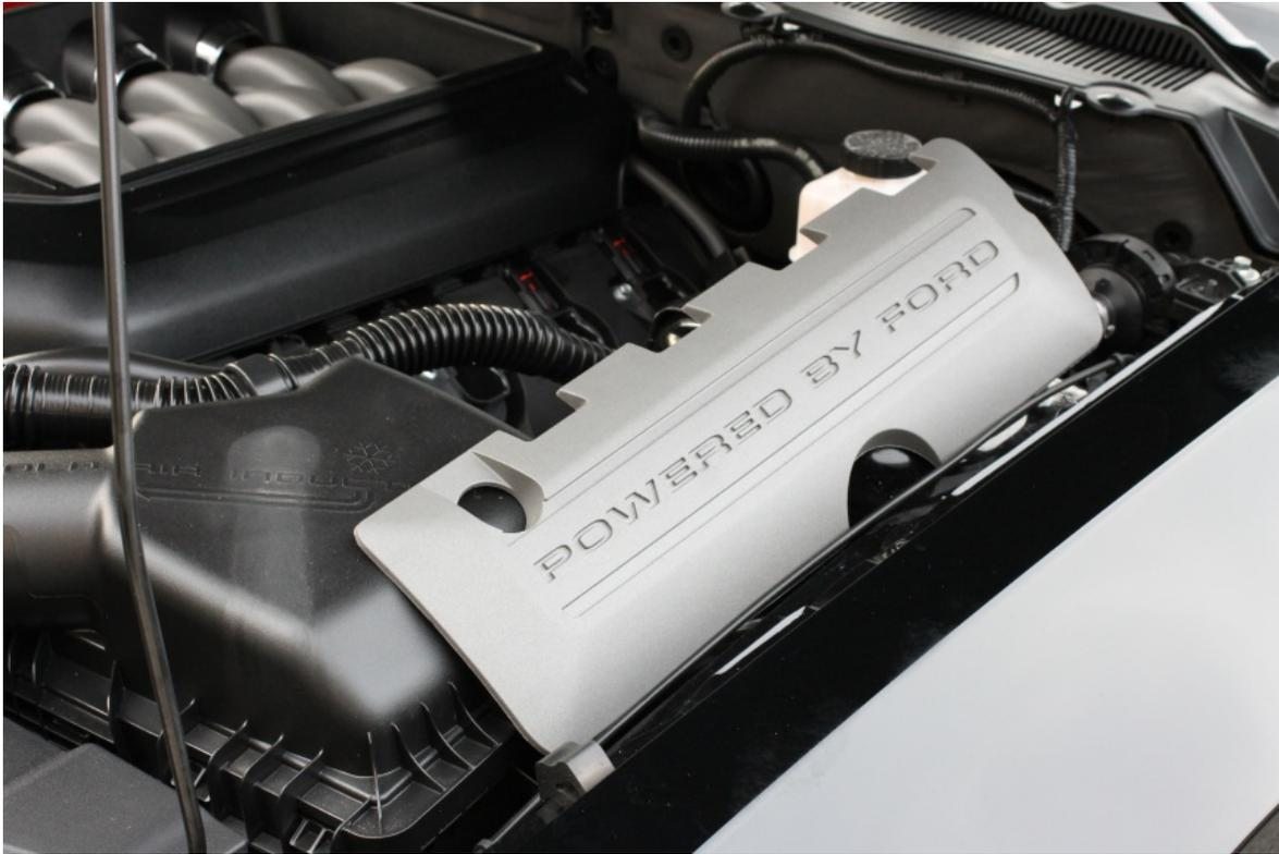
9. Slide the correct Boss 302 Coil Cover into position, and press firmly to lock it into place – replace the PCV Tube.
