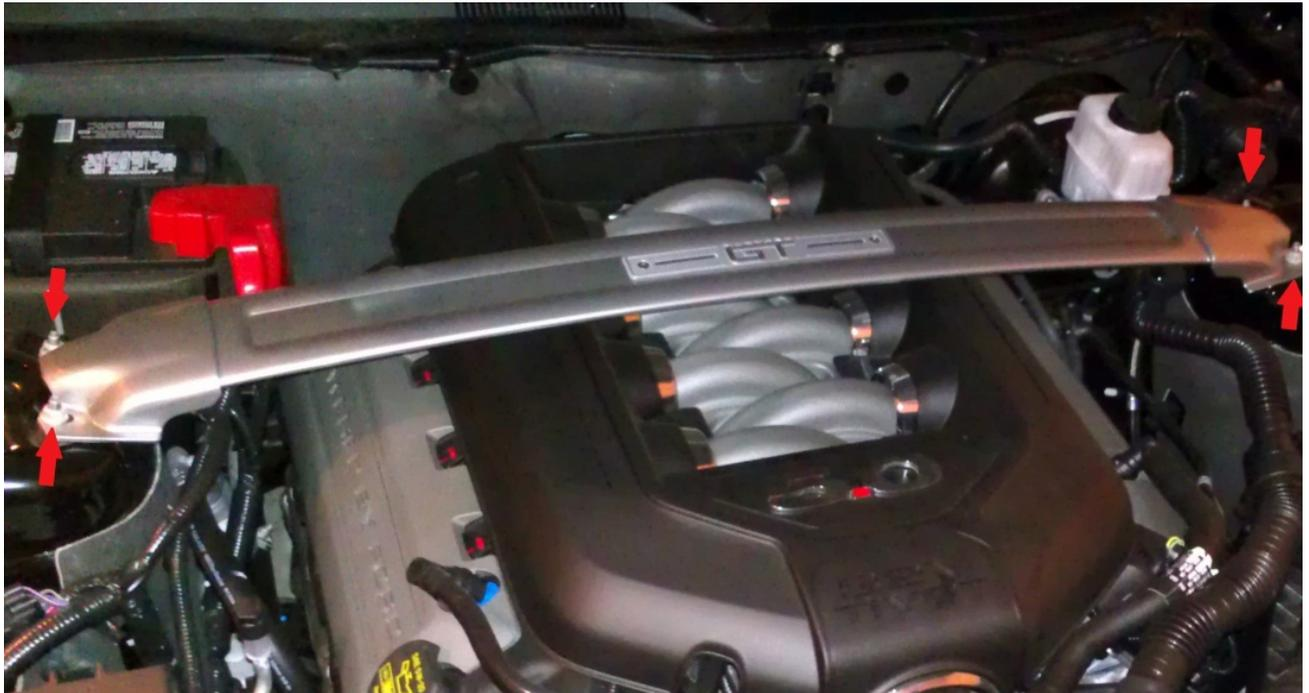
2. Remove your **Intake Cover** simply by pulling up on the cover and unsnapping it.
