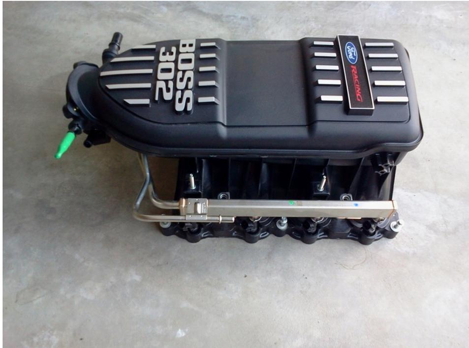
Finger tighten the 6 **Intake Manifold retaining bolts** and the 4 **Fuel Rail retaining bolts**, then torque them to **89 inch-pound** in the following respective sequences:
