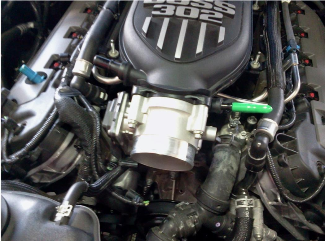
17. Get your (2) **Pliers** and **Friend** back and reinstall the **Brake Booster Vacuum Tube** to the Port on the **LH** front of the **Intake Manifold** just below the **Green Cap** pictured and ensure it isn't kinked.
