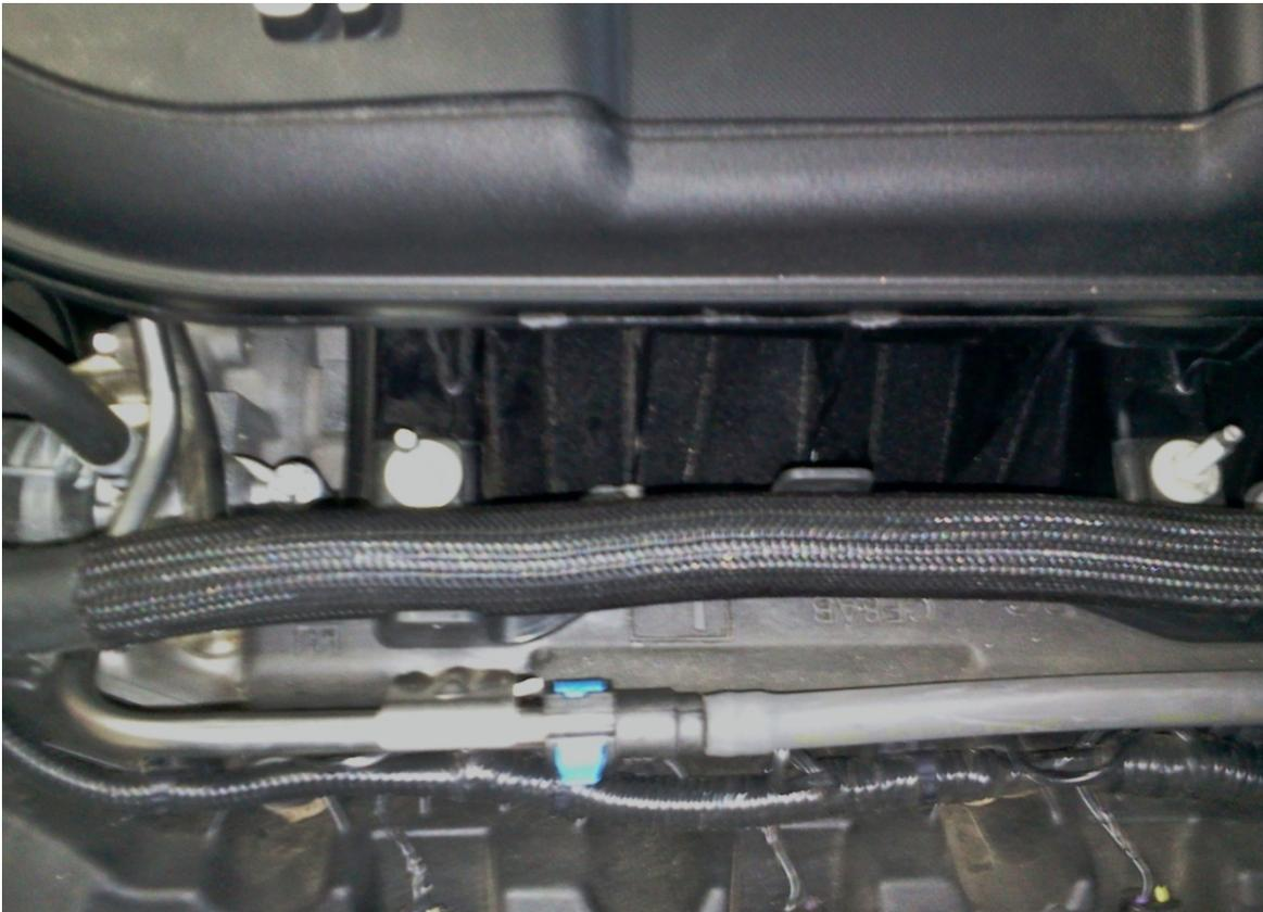
16. Reinstall the **Throttle Body** with the (4) **bolts (8mm)** along with its **electrical connector**.
