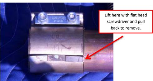
7. You will also need to reuse the stock clamps from the converter side of the H-pipe for the new X-pipe. I just bent each clamp back and forth until the tab broke. Repeat on other side.
