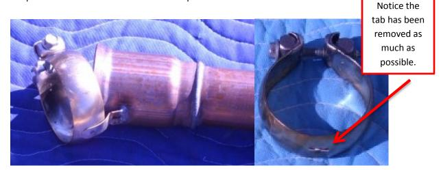
8. Now, gather your factory clamps and new Ford Racing X-pipe. Slide the rear factory clamps on the rear midpipes.
