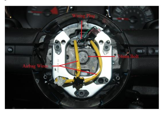
9. Plug in and reinstall airbag assembly using the two 8mm bolts, then plug holes with plastic caps
