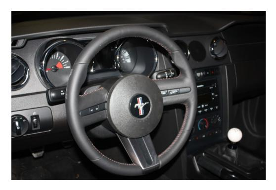
9. Reconnect battery and test horn and turn signals for correct operation.
