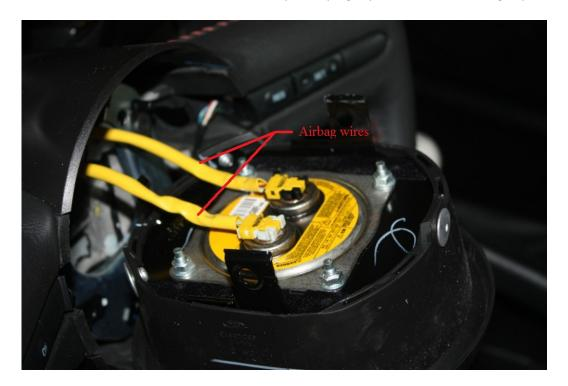
4. Remove wires from the airbag and place airbag in secure location to avoid damage. (Airbag to be used with new steering wheel)
