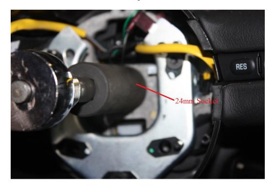
7. Remove stock steering wheel being careful not to damage airbag wires. (No wheel puller required)
