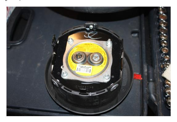
5. Unplug steering wheel wiring harness using the needle nose pliers.
