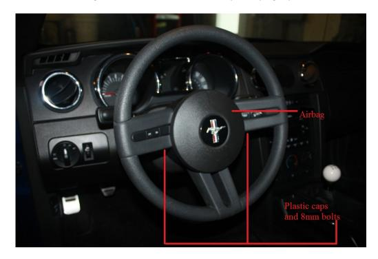
3. Remove the (2) 8mm bolts that are found under the plastic plug caps that hold the airbag in place.
