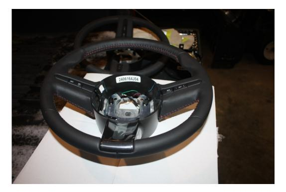
8. Now install the new steering wheel and feed the two yellow coated wires through the hole in the base of steering wheel.
