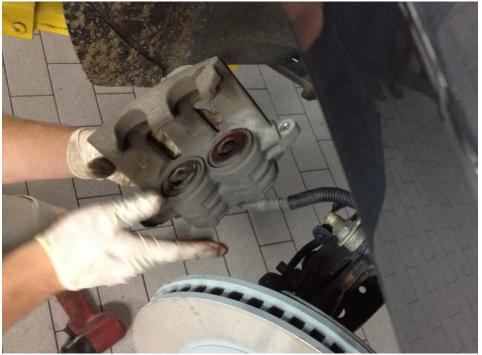
14. Reinstall the caliper over the new brake pads. These should slide in place with perhaps a little persuasion. They will bolt into the caliper bracket using the bolts you set aside earlier.
