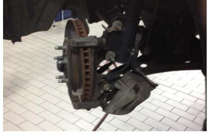
7. Next, you must take off the old Caliper bracket. This is very similar to taking off the caliper. Just 2 bolts in back of the piece and it's out.
