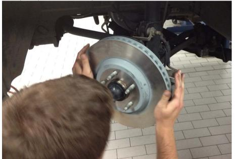
10. Attach your new Caliper bracket with the same bolts and holes you removed the old one with.
