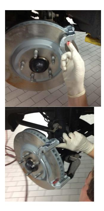
12. Install new Brake Pads in the caliper brackets. Once again both sides. Make sure the "friction side" is towards the rotor.
