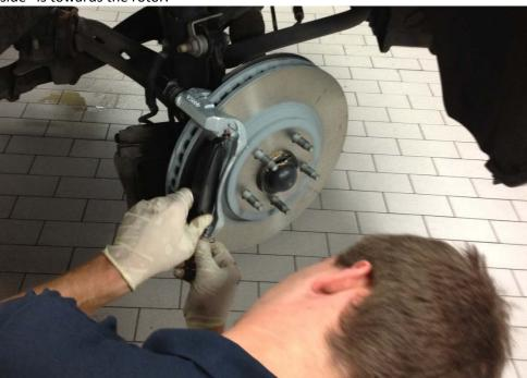
13. Apply Grease on the caliper where it comes in contact with the brake pads. If you apply it to the pads themselves, you will see the grease on the back of the pads whenever you look at your brakes.
