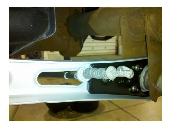
14. Seat the end of the emergency brake cable in its seat.
