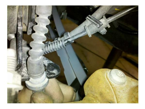
16. Replace the clip in the collar of the emergency brake cable.
