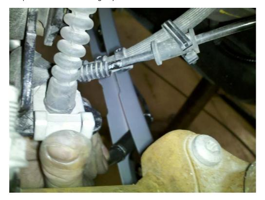
17. Reinstall the emergency brake cable bracket.
