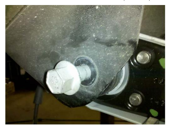
11. Using a torque wrench with an 18mm socket, torque rear bolt to 129 ft-lbs.
