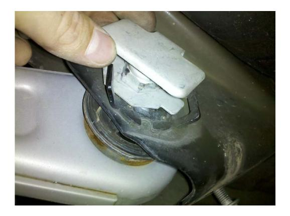
6. Using the 18mm wrench, remove the rear bolt from the control arm. The nut on the rear bolt has a handle; you may need to use your other hand to hold this while you remove the bolt.
