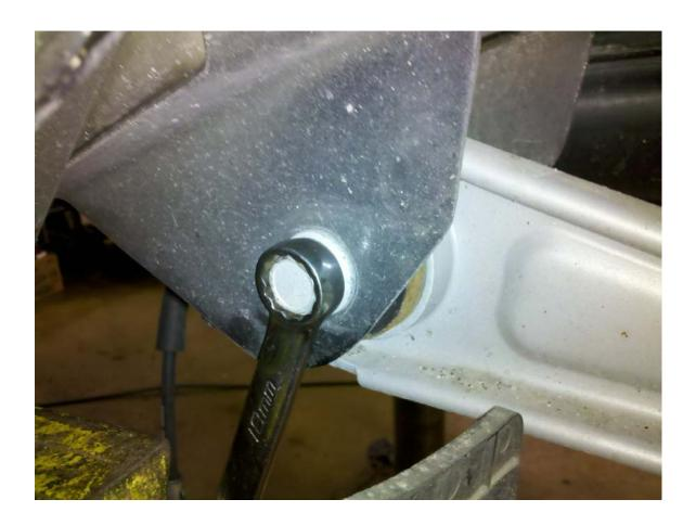
5. Once the bolt is out, the nut will still be in place. Rotate the nut clockwise to remove it. **NOTE:** This nut will not be reused and can be discarded.
