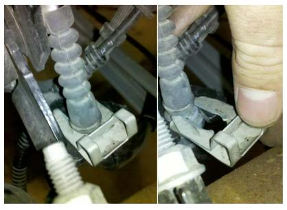
3. Remove the end of the emergency brake from the bracket and then feed the cable through the LCA.
