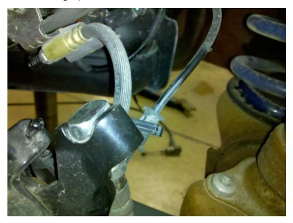
15. Reinstall the base of the emergency brake into its position on the caliper bracket.
