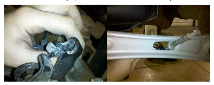
4. Using the 18mm wrench, remove the front bolt from the control arm. **NOTE:** This bolt will not be reused and can be discarded.
