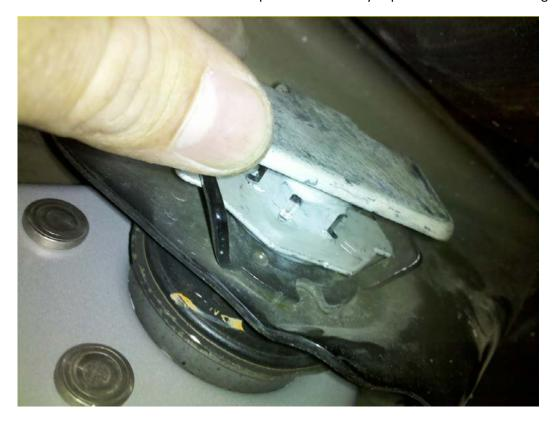
10. Insert the new front bolt into the front bushing of the control arm from the outer side of the car toward the center of the car. You will be able to thread it into the new nut with tabs placed in the previous step.
