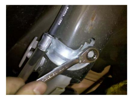
2. Locate and remove clip holding the emergency brake cable to the caliper bracket. **NOTE:** Keep clip as it will be reused.
