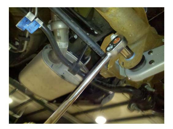
12. Using the same torque wrench and 18mm socket, torque the front bolt to 129 ft-lbs.
