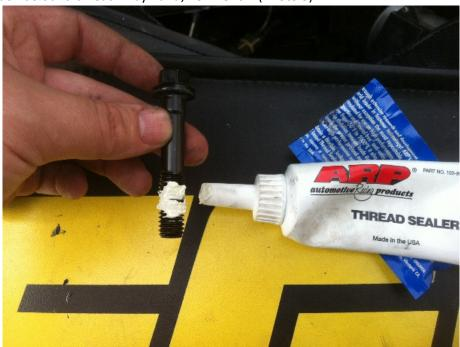
Photo 3. Applying thread sealer for the short bolts that will be in the water jackets.
