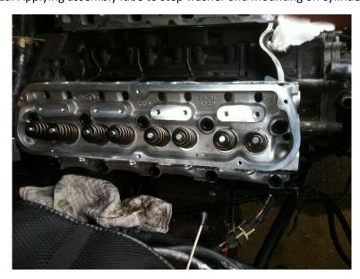
Photo 1b. View of all step washers in place on cylinder head.
