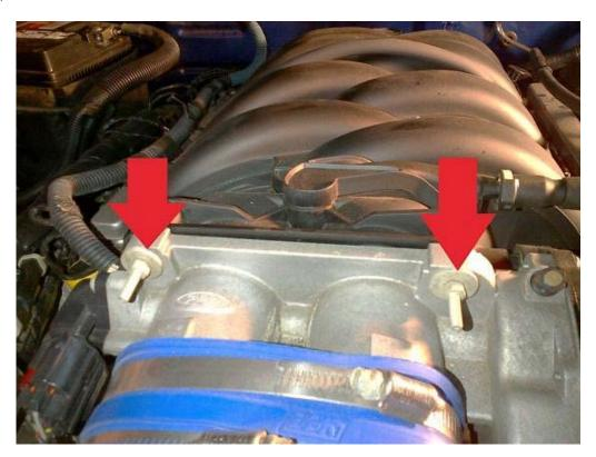
If you DON'T see these bolts sticking out and instead just see a normal bolt head, then you'll need to go out and buy (2) new bolts with the protruding ends before you can continue. You can remove (1) of the back bolts removed in Step 2 to take with you to the auto parts store for reference.
