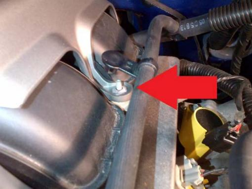
5. You don't need to do anything further at the front, but at the rear, make sure you reattach the black plastic clips after you've installed the engine cover.
