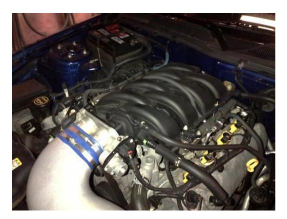
2. The intake cover installs relatively easily. At the rear of the engine on <u>both sides</u>, you'll need to pry off the black plastic clip attached to the bolt shown in the picture. This is right beside the fuel rail.
