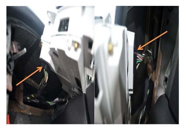
8. Now your gauge cluster can be removed and taken to a table to remove the rest of the screws.
