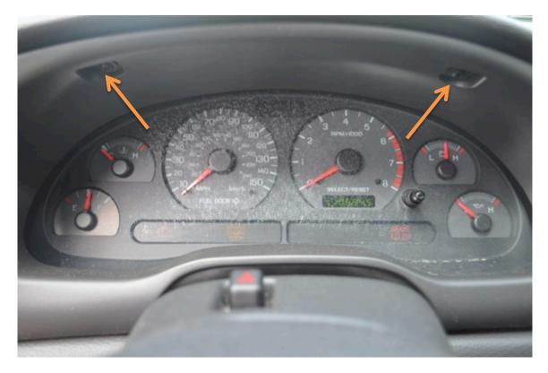
4. Now the panel should remove by pulling straight out. Do this carefully so you do not break the clips behind it.
