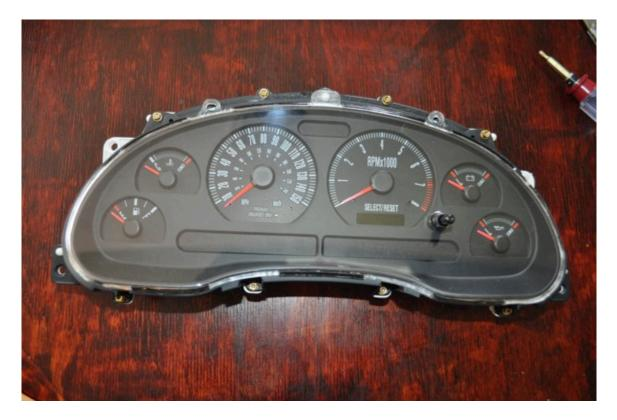
**12.** Now re-install your gauges back into the car. Remember to connect both harnesses securely and then mount the gauges back in using the four black t15 torx screws. Also make sure to turn the car on to check and make sure the gauges work.
