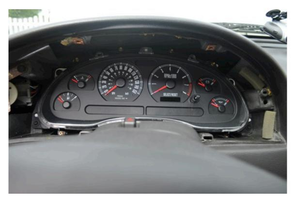
**13.** Next install the cover by popping it into place and screwing the two remaining black t15 screws into the top. Then put your headlight knob back on.
