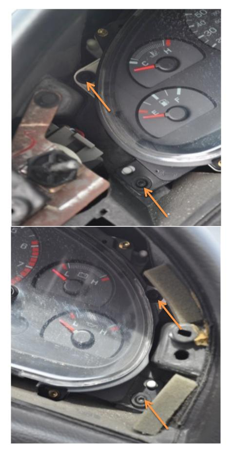
**6.** Now begin to pull the gauge panel straight out while tilting it back. There are two harnesses connected to the back. One on the left side upper and one on the left side upper, remove these and the gauge panel will come out freely.
