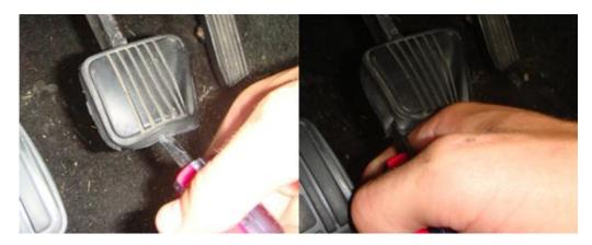
4. When you're ready to install the new one, you're going to want to put the right side of the cover on first, by sliding it into place.
