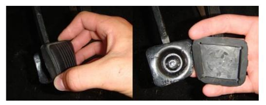
5. Next, bend the top rubber clip over the pedal, followed by the left clip, and finishing with the bottom clip. Push on the cover until you are satisfied with how it is sitting on the pedal, and finish with sitting on the seat and pushing on it with your foot in order to test it out.
