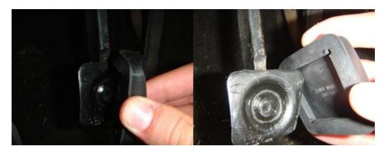
6. Next, bend the top rubber clip over the pedal, followed by the left clip, and finishing with the bottom clip. Push on the cover until you are satisfied with how it is sitting on the pedal, and finish with sitting on the seat and pushing on it with your foot in order to test it out.
