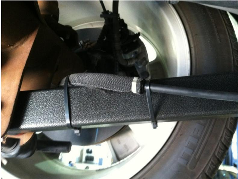
8. Give each grease zerk a couple pumps with a grease gun, if you don't have access to a grease gun, go buy one, you will use it in the future and will keep the mounts quiet and happy.
