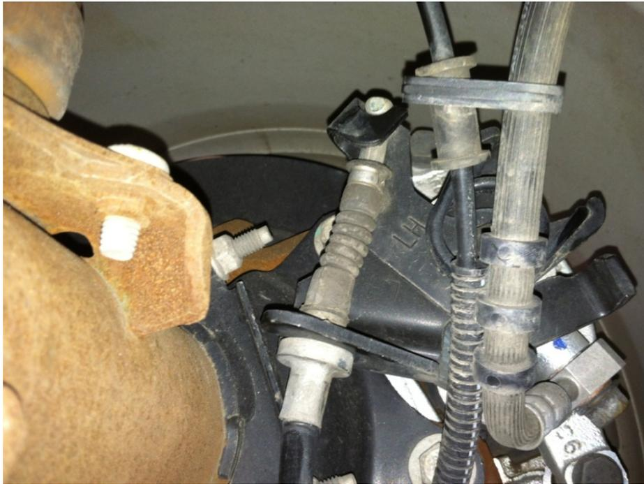
4. Use the 18mm to unbolt either end of the LCA, it will swing down so stay clear. Remove the second bolt holding the other end of the arm and move it off to the side.
