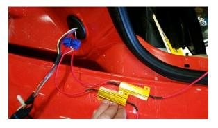
**STEP 5.** Using the other two supplied wire splice connectors, wire the other side of the load equalizers to the ground circuit.
