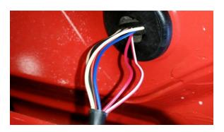
**STEP 4.** Using the supplied wire splice connectors, wire one side of each load equalizer into each signal wire.
