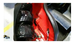
**STEP 3.** Identify the signal wires (red / white) and ground wire (black) after the harness connector.
