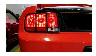
\*Note the bulbs are can be installed into the socket, but will only functions one way. If they do not turn on, flip the bulbs 180 degrees and retest.
