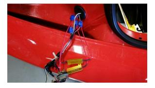
**STEP 6.** Install the LED bulbs into the factory harness and reinstall the taillight housing to the vehicle.
