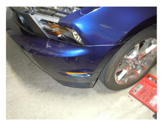
11. Remove the two 8mm bolts from the top of the grill, lift the cover off the tabs beside the bolts and rem the bumper cover.
