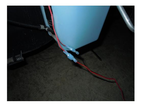
49. Turn on the parking lamp switch to check the electrical connection. If the lamp does not turn on, turn o switch and proceed to check your crimps for continuity with the wire. If the connections are sound, try switch again until the light turns on.
