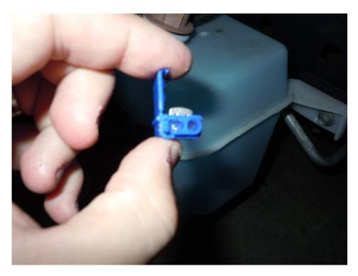
42. Fold the  $\frac{1}{2}$  of stripped red wire over the insulation.
