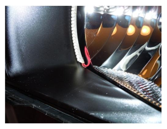
30. Remove any sealant from the headlamp cover with a screwdriver and the heat gun.
