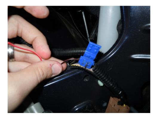
43. Insert it into the splice and close the blue cover. It may be necessary to use a pair of pliers to close the c
