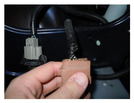
38. Use a knife, scissors, or a pair of snips to remove a portion of the wire routing.
