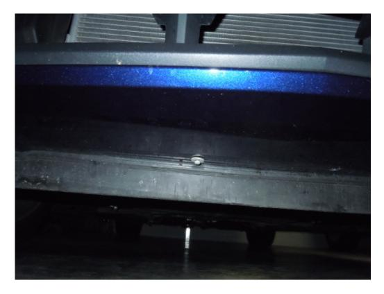
5. Remove the (5) 7mm bolts from the air dam under the car.
