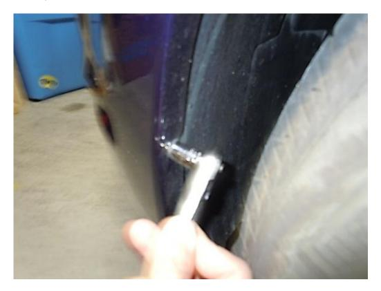
4. Remove the (4) 7mm bolts from the air dam in the front.
