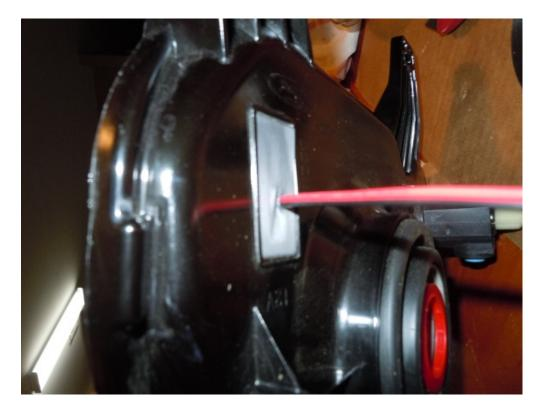
29. Insert the inner cover back into the housing. Route the wiring through the hole in the seal. Route the w
