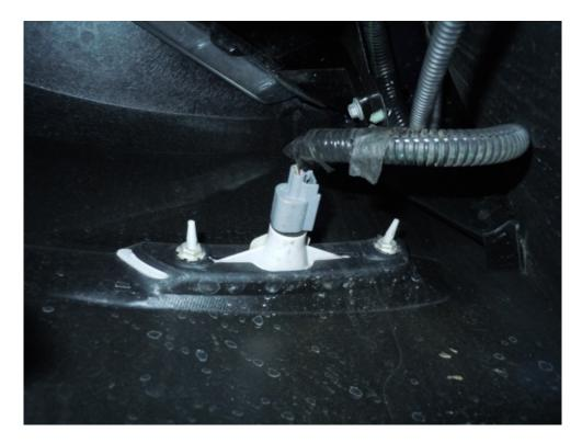
8. Remove or unplug the ambient air temperature sensor in the front valence.
