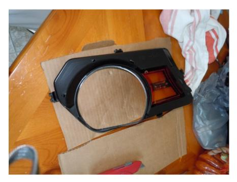
23. Remove the Oracle Halo unit from its wrapping. Test the LEDs using a 12 V power source. If faulty conta American Muscle or the manufacturer. Line up the ring with the back edge of the cover.
