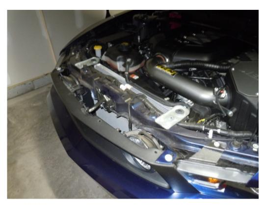
3. Remove the 4 splash shield screws (2 each side) with the 7mm socket.
