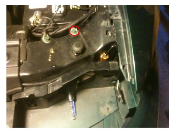
\*The ground side can be connected to the ground black wire running to the turn signal bulb\*
