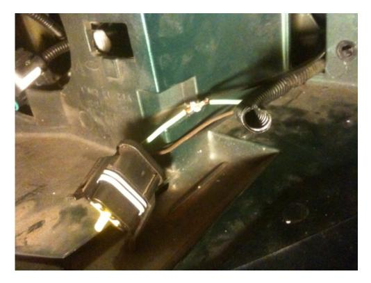
7. After the solder has cooled, tape the connection with electrical tape and replace the plastic wire protector cover. Put the turn signal bulbs back into the headlamp and turn clock wise till clicks into place. Reconnect the headlights and turn signal connectors. Before putting the headlamps all the way back in, test the LED's.
