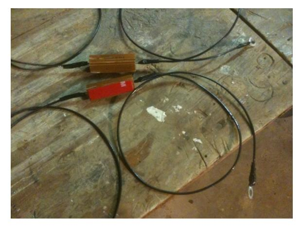
5. I placed the resistors behind the head light bracket using the 3M tape. I ran the wires through the framing and behind the fender using holes drilled from the factory. I connected the ring terminals to factory green ground bolts located on the frame.
