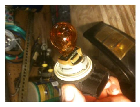
3. Remove the bulb by pulling straight out. Then take the new LED bulbs and replace by sliding straight into the socket
