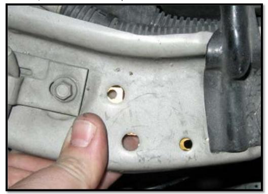
♦ With a flat washer on the head of the screw, install them using a Nylon locking nut on the bottom side.
