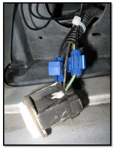
♦ For added protection, wrap electrical tape between the tubing and the lamp socket
