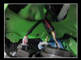
STEP 8: Connect the factory wiring harnesses to your new headlight and install onto vehicle. Use the same 10mm bolts removed in Steps 1 & 2 to secure the headlight to the vehicle. Repeat steps 1-7 for opposite side. Be sure to check the functionality of all lights before re-installing the bumper cover.
