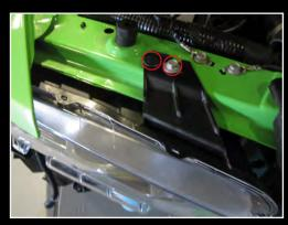
**STEP 1:** With the bumper cover removed, remove the plastic retaining clip and 10mm bolt on the top of the headlight housing as shown.
