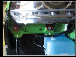
STEP 2: Remove the two 10mm bolts holding the lower portion of the headlight housing to the bumper support. Pull the headlight away from the vehicle and disconnect the two wiring harnesses as shown. You can now remove the headlight from the vehicle.
