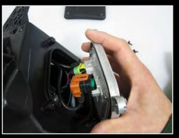
**STEP 4:** Disconnect the two wiring harness clips once the ballast is loose from the housing and set it aside (It will be re-used on the new head).
