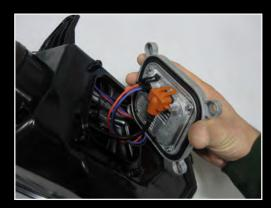
**STEP 7:** Route the HID bulb harness through the housing so it can be connected to the ballast.
