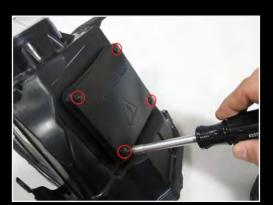
**STEP 3:** Lay the factory headlight next to the new headlight on a workbench, taking care to not scratch the lens on either light. Using a T15 Torx Bit, remove the factory HID ballast from the headlight as shown.
