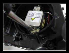
**STEP 5:** Remove the bulb cover on the factory housing to expose the HID bulb. Use a Phillips Head Screwdriver to release the bulb from the housing. Also remove the small wiring harness that goes from the HID bulb to the HID Ballast, it will be re-used on your new headlight. Note: Never touch the HID bulb itself with your fingers.
