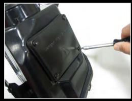
**STEP 7b:** Connect the two wiring harnesses to the factory ballast and install the ballast onto the new headlight housing using the T15 Torx head screws removed from the factory housing in Step 3.
