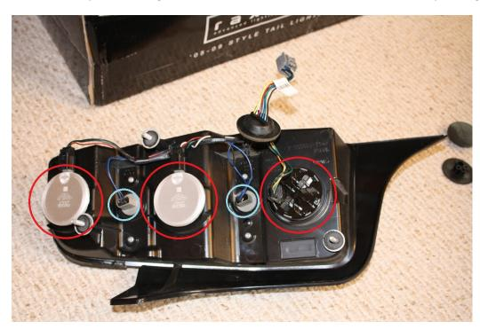
8. Install the harness and bulbs into the new taillights. Note that on the new taillights, the reverse bulbs are at the bottom of the assembly:
