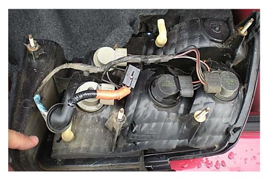
9. Remove the bulbs from the factory harness and insert them into the new sequential harness.
