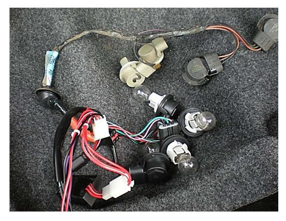
10. Re-install the sequential harness into the taillight assembly. Plug the lights in before reassembling the taillight to ensure you have the correct sequence. This will make for less work if installed in the wrong sequence.
