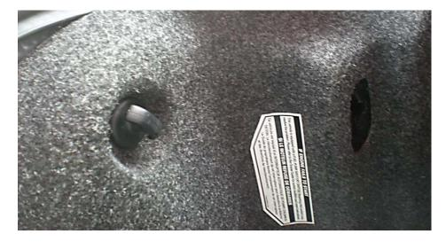
4. Remove both the front liner and back liner so you can move the liners on both the left and right sides to access the tail light assembly bolts.
