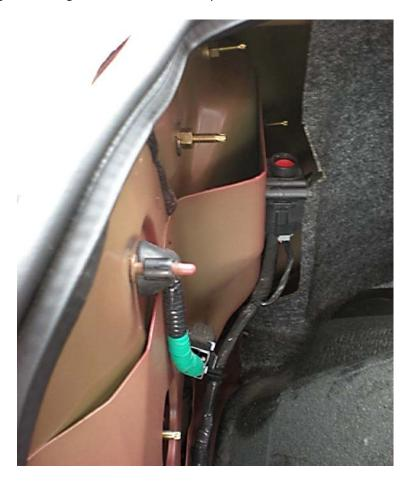
6. Unplug the factory light harness and dismount the rubber grommet by pushing it through a little bit at a time. A screw driver may help with this step.
