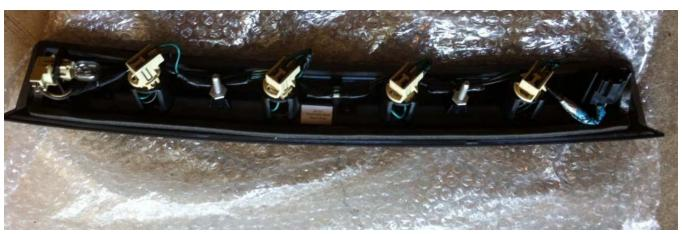
7. Your harness work is done now. Proceed to reinstalling the new brake light into the deck lid/trunk. Connect the wiring harness from the trunk to the new brake lights. Make sure all your lights work. (see below). Reconnect the two 10mm bolts.
