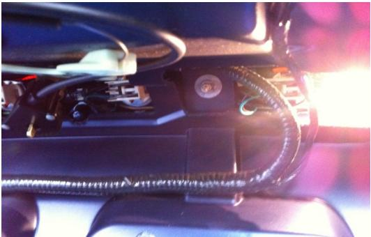
2. On the driver side, press the clip in on the wiring harness and pulling. Be careful with this step as the older plastic is very easy to break.
