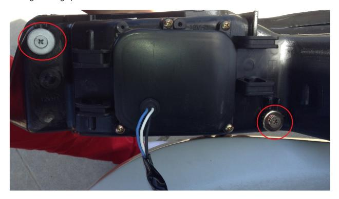
To adjust the vertical alignment of the light intensity to your preference, use a screwdriver to turn the silver screw. Pulling out the headlight will possibly be necessary.
