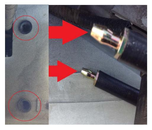
When you see the black insert where the pins are put in, you can insert the pins to secure the headlight.
