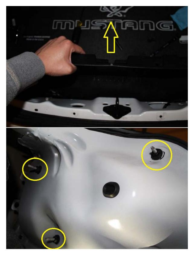
4. Use your 11mm socket wrench to remove 3 nuts holding the tail light to the vehicle.
