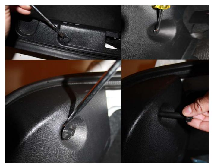
3. Remove plastic trim cover and locate 3 nuts holding each tail light to the vehicle.
