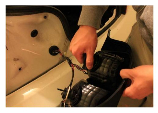
\*\*Using gloves to handle the bulbs is optional, just make sure you do not touch the glass bulb itself as your natural body oils may heat up on it, causing your bulb to burn out faster.\*\*
