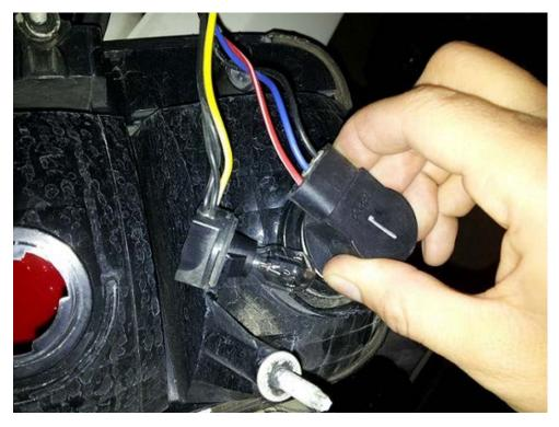
7. Replace the light bulbs into your new tail light housing, turning clockwise.
