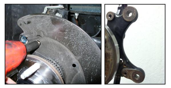
Figure 1: Removal of dust shield (passenger side)
