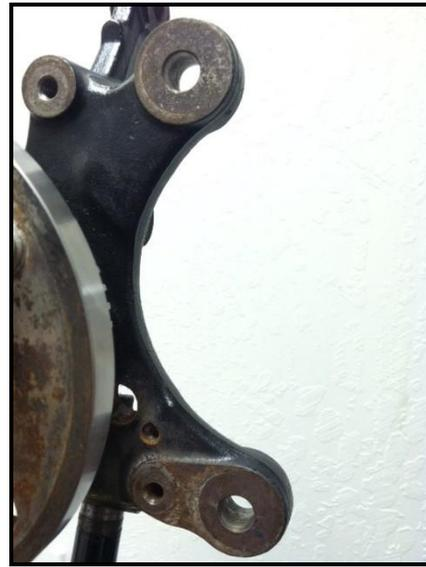
**Figure 2:** OE caliper mounting surface (driver's side)
