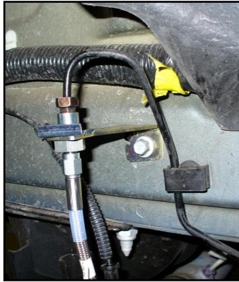
**Figure 5:** Brake hose attached to hardline
