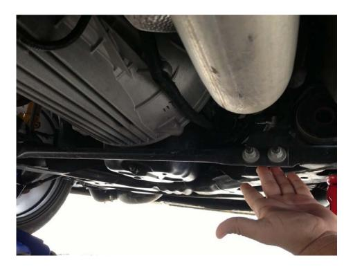
3. Using a 15mm Deep Well Socket, remove all the nuts holding in the front brace. Remove the brace and store it. It will not be reused.
