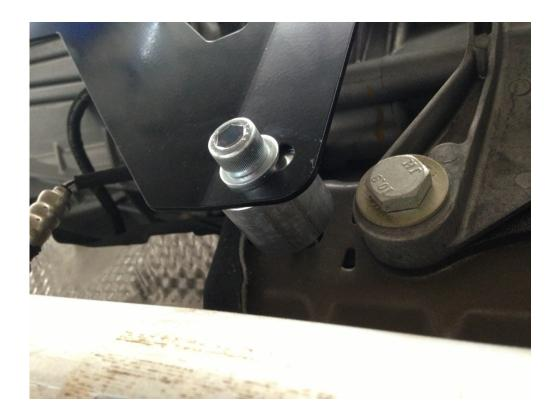
7. Using an H10 socket, tighten the back bolts. Tighten it using a ratchet.
