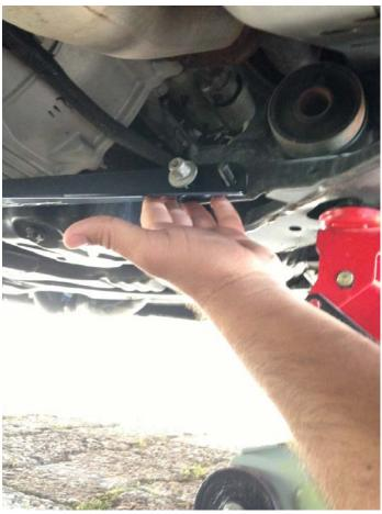
4. Place the new Hotchkis brace over the studs were the old brace was. Using the nuts you removed, put them back on but do not tighten at this time.
