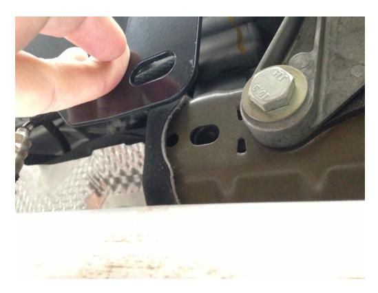
6. Place a spacer in-between the car and the brace, then using the supplied bolts and washers to mount the brace onto the car.
