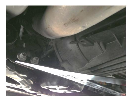
5. Using the new brace as a guide, find the holes where you will bolt in the new brace.
