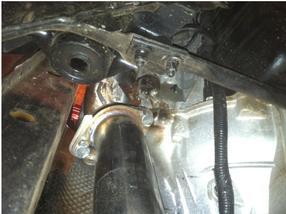
New cat-delete pipe in place attached to manifolds
