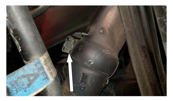
• Loosen this bolt shown above for both the passenger and driver side resonators. These will not be reused again.
