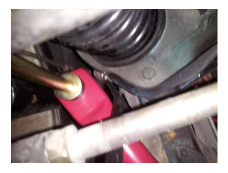
**12.** Smile, the hard part is over! Now that the second end link is installed, it is time to torque down all the bolts! According to my Chilton's manual, the end link torque specs are "8-12 ft. lbs. (12-16Nm). I personally, torque them to 14 ft. lbs. Do what you wish, and ALWAYS double check torque specs to sources that you trust.
