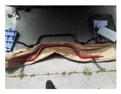
**6.** Now it is time to take off the brackets for the bushings, you will need these as Eibach has only given you the bushings and not the brackets. This is actually very simple, just take a flat head screw driver and pop the top off.
