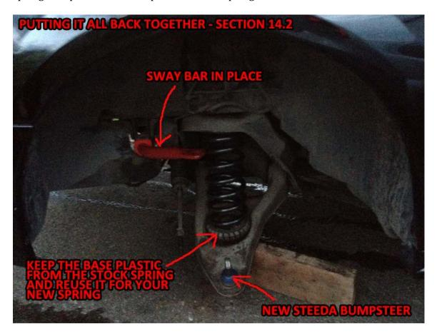
14.3 – With the spring in place properly placed put a jack under the metal triangle and push up to compress the spring into place.
