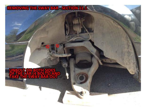
11.2 – Take the sway bar out of the car and unclip both supports from the sway bar. Discard the plastic bushings.
