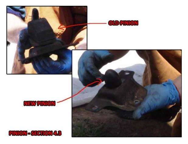
4.4 – Replace the pinion assembly back under the car and bolt the 3 screws with a  $12\ \mathrm{mm}$  wrench.
