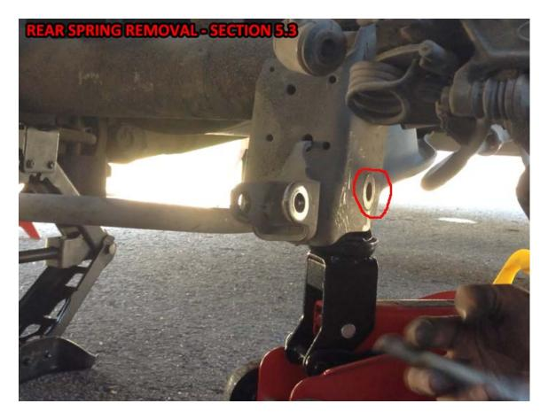
5.4 – Use the jack to slowly lower the metal bar and take out the spring. Note the position of the spring.
