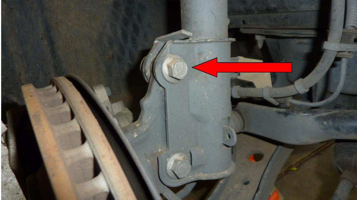
6) Use your 18mm socket to loosen the top strut bolt. You will see that the bolt will turn and so will its clip from the other side of the spindle. This will spin until it binds up with the rest of the spindle. It will then loosen as you spin the bolt.
