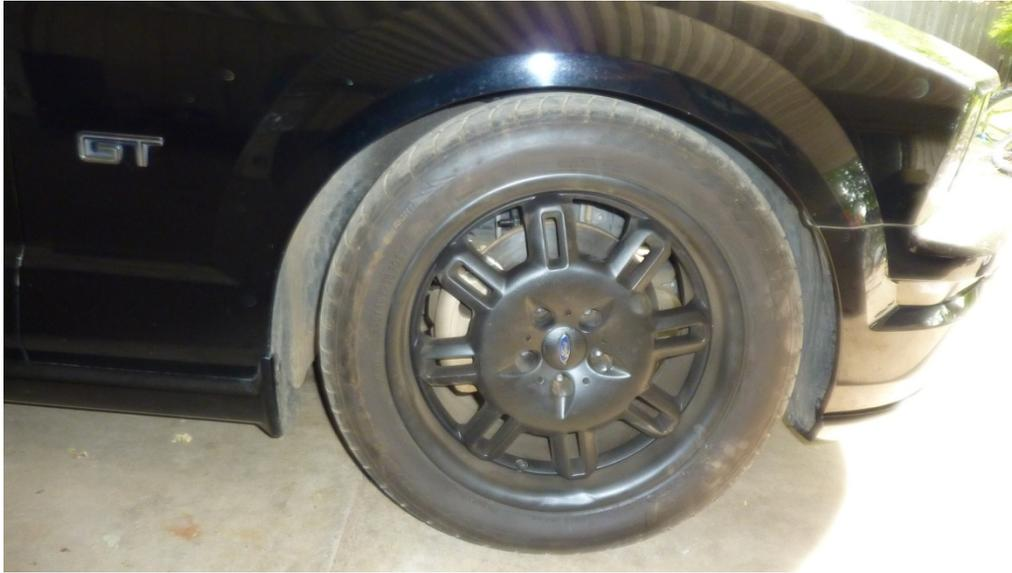
12) When re-installing your tires, make sure you tighten each of the lugs nuts to at least 100 ft/lbs of torque to insure your safety and that your wheels will stay on while in motion.
