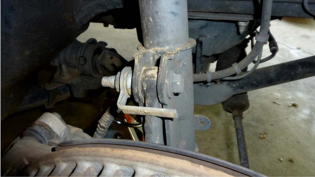
7) Remove the top strut bolt and prepare to install the camber adjustment bolt.
