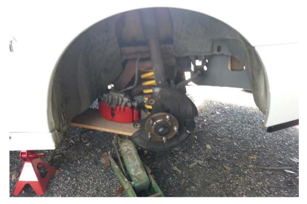
3. Remove the top bolt that holds the strut to the spindle, and loosen or remove the nut from the bottom one. (Do not remove the bottom bolt completely, or the control arm will drop, and the spring will violently decompress.)
