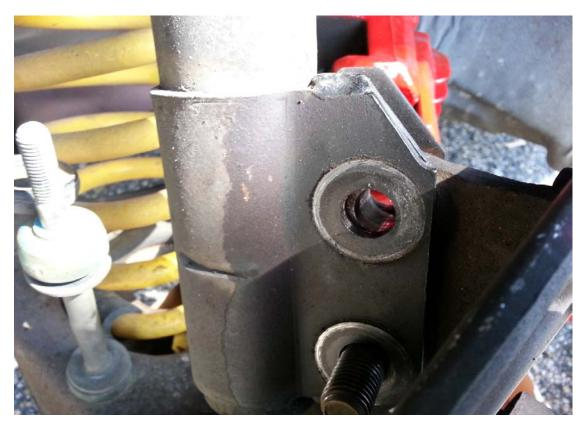
4. Your new camber bolt has a cam lobe that pushes the top of the spindle toward or away from the strut. To correct for the usual negative camber, we want it to push the top of the spindle AWAY from the strut, as shown in the above photo.
