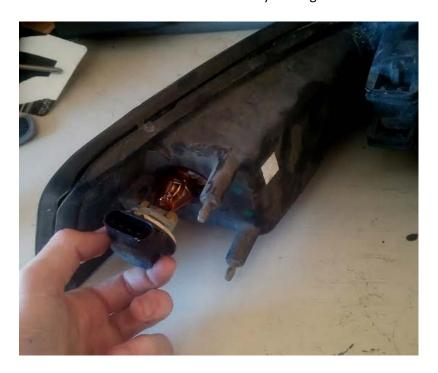
7. Place the new housing on your workbench and install the blinker by screwing it in clockwise.
