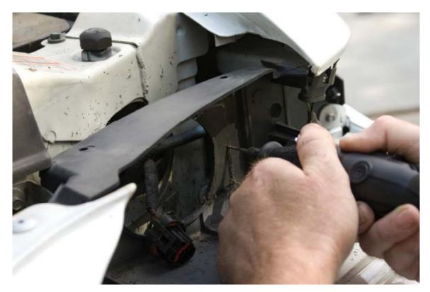
9. The finished cut should look as shown. Test fit the new headlight assembly and ensure there is no interference. Once complete and everything fits fine, remove the plastic shavings, if there are any.
