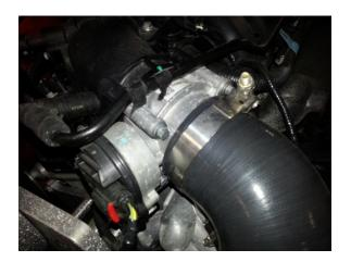
3. Place the supplied gasket between the throttle body and the spacer.
