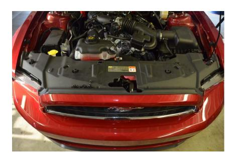
2. Remove the (4) Phillips head screws and the (4) 8mm bolts under the radiator cover.
