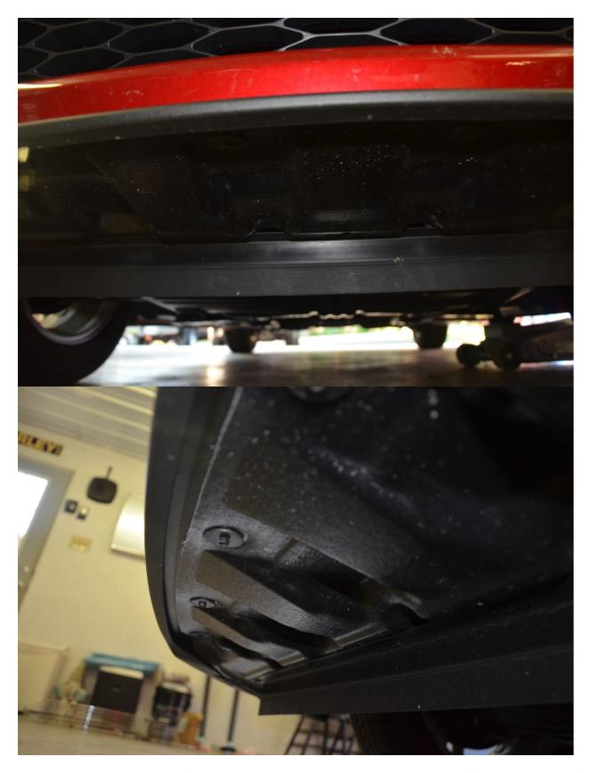
5. Making sure everything is out of the way and having your sheet ready gently pull the front bumper away from the car, there are tabs that will release and create a loud cracking sound. This is perfectly natural and nothing to worry about.
