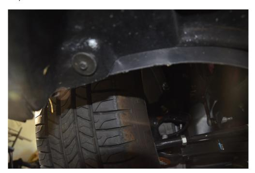
4. Remove the (12) 7mm bolts from the outer lip of the air splitter; this will basically release the bumper from being attached to anything other than the clips holding it to the quarter panels.
