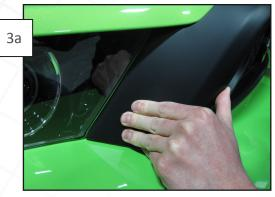
Beginning with either side of the bumper, place the blackout flush up against the headlight, making sure that the front edge is flush with the grille.
