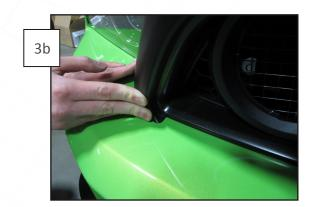
Once the part is properly aligned, press down firmly to fully seat the tape.
