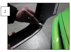
Peel the back from the 3M Adhesive Tape as shown.
