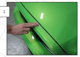
Using the supplied alcohol prep pad, thoroughly wipe down the area of the front bumper surround to which the grille blackout will adhere.
