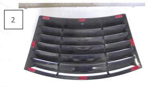
Lay the louvers upside down on a surface that will not scratch the finish. Install the 8 brackets as shown and install the nuts finger tight. You just want to tighten the brackets enough so they stay in place; there is no need to fully tighten them at this point.
