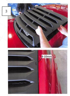
Peel the backing from the adhesive tape on the brackets and apply some of the 3M Adhesion Promoter to the tape. Using a partner, place the louvers over the rear window aligning the tape edge of the louver with the tope edge of the rubber strip around the rear glass. There should be 8-10mm between the louver and the C pillar on each side as shown in the photo above.
