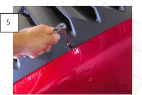
Once the sealant has cured, install the louver onto the brackets using the supplied washers and closed end nuts. Use an 8mm socket and ¼ drive ratchet to install the nuts just past finger tight. Do not over tighten the nuts as you will risk damaging the studs.
