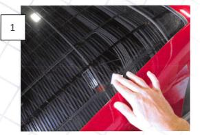
Using the supplied alcohol prep pads, wipe down the outer edge of the glass where the brackets will adhere. Once the alcohol has dried on the glass, repeat this process using the included 3M Adhesion Promoter.
