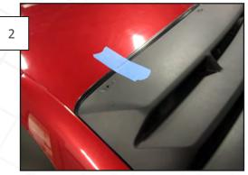
Place the louvers over the rear window, centering them left to right and lining them up with the edge of the upper weatherstripping. Once properly aligned, tape the upper corners of the louver to the car using either painters or masking tape as shown.
