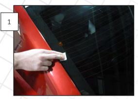
Using the supplied alcohol prep pads, wipe down the outer edge of the glass as shown. Repeat using the included 3M Adhesion Promoter as well.
