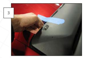
Remove the nut/washer from the plate, peel backing from tape, then slightly lift upper corners of the louver to insert the stud through the mounting hole as shown. Making sure the louver is still properly aligned, firmly press down to fully seat the adhesive tape. Repeat this step for the remaining 6 plates. You can remove the tape applied in Step 2 at this point.
