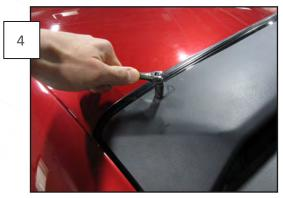
Once all eight of the plates are installed and secured to the window, place the washers over the studs followed by the nuts and tighten with an 8mm wrench or socket. This completes the installation of your rear window louvers. *Cleaning: To clean your rear window, simply remove the 8mm nuts/washers and remove the louver from the vehicle.*
