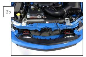
Be sure to unplug the two wiring harnesses for the fog lights before removing the grille assembly.
