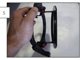
Install the fog light delete in the bracket by placing one end over the post and sliding the other end down over the clip as shown above.
