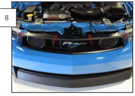
Re-install the grille assembly into the front bumper cover by simply pushing it back in and letting the clips seat themselves. Re-install the plastic radiator cover to complete the installation.
