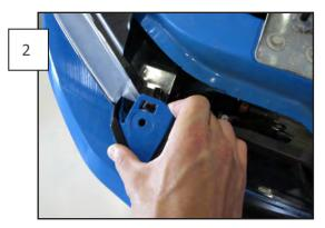
Pull the bumper cover over the locating tab as shown. Then, using a flat head screwdriver or trim removal tool, gently pry back the tabs on the factory grille and pull it away from the bumper cover. Start on the outside tabs then pull the grille away from the bumper cover as an assembly.
