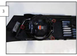
With the grille assembly removed, unbolt the four 7mm screws for the fog light mounting bracket and remove it from the grille.
