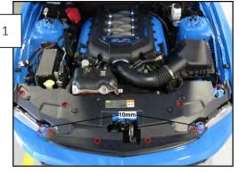
Remove the 8 pins securing the plastic radiator cover and remove it from the vehicle. Also remove the two 10mm upper bolts for the bumper cover.
