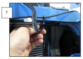
Repeat Steps 3-7 for opposite side fog light. Once both fog light deletes are installed in the grille assembly, find a safe place to secure the factory wiring harnesses.
