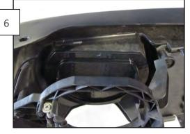
Re-install the fog light bracket into the grille using the 3 7mm screws removed in Step 3. Make sure the fog light delete is flush against the opening in the factory grille as shown.
