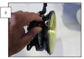
Remove the fog light from the mounting bracket by pulling the tab back as shown above.
