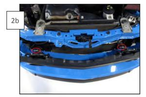
Be sure to unplug the two electrical connectors for the fog light bulbs before completely removing the grille assembly.
