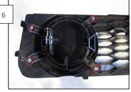
Re-install the fog light bracket to the grille assembly with the 4 screws removed in Step  $\bf 3$  .
