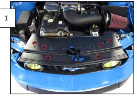
Remove the 6 pins securing the plastic radiator cover and remove it from the vehicle.
