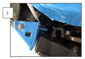
Using a flat head screwdriver or trim removal tool, gently pry back the outer tabs securing the grille to the bumper support and remove it from the vehicle. Begin with the outside tabs, once they are loose, the grille can be pulled straight away from the vehicle
