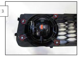
With the grille assembly removed, unbolt the four 7mm screws for the fog light mounting bracket and remove it from the grille (Some vehicles use Phillips head screws for the fog light mounting brackets).
