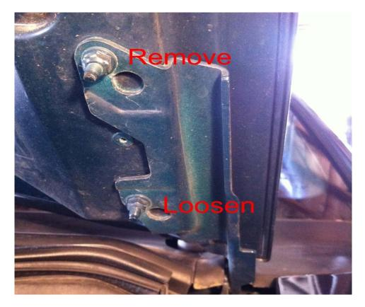
5. Slide the slotted end of the top (larger) bracket on the loose nut. Position so the top stud lines up with the hole in the bracket, reinstall top nut and tighten both.
