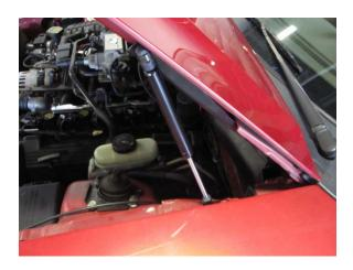
Repeat Steps 1-4 for opposite side strut assembly. You may remove the factory prop rod at this point. Be sure to close hood carefully after installation to ensure proper alignment of hood. If any adjustment is needed, the mounting holes in the strut brackets are slotted for easy alignment.
